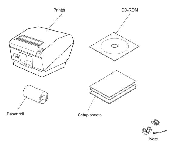
**Note:** The ferrite core and fastener provided with your printer depend on your printer configuration.
